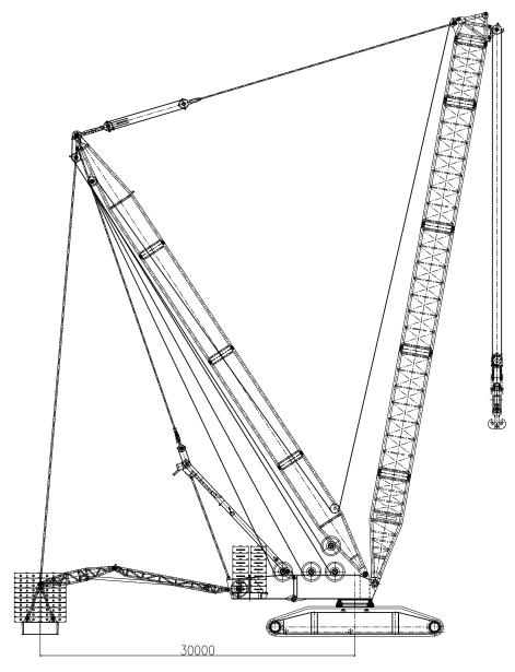
1.2 Overall dimension under superlift heavy-duty jib working conditions
